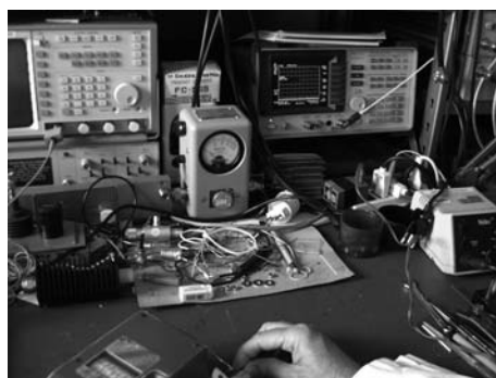
Fig. 3. A) Experimental asset. The far-field spectrum analyzer is placed on the table about 50 cm. far from the g.d.m and the passive oscillator. A small antenna picks up the r.f. field. The author right hand is moving the L/C oscillator tuning to achieve a resonance with the grid dip meter: when the resonance is achieved, the spectral line on the display is immediately depressed (B)
